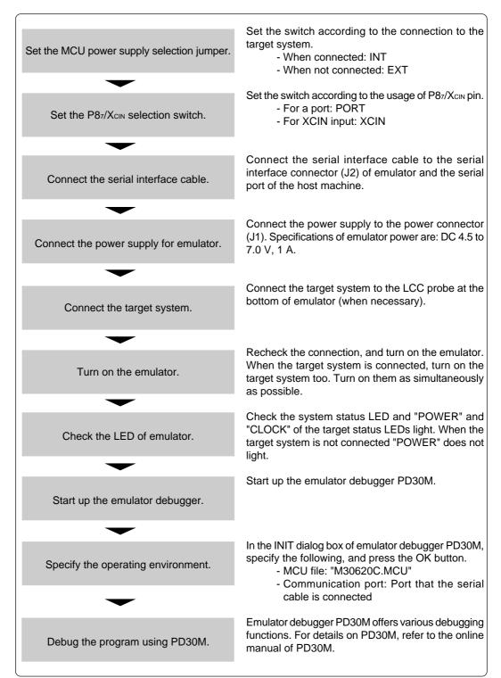
Figure 2.3 Procedure for starting up the emulator
